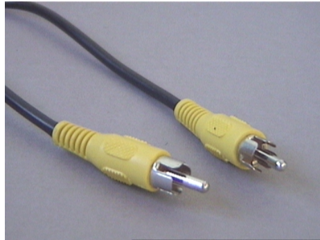
fig. 4: Use this cable to connect a device with a Video-Out port.
