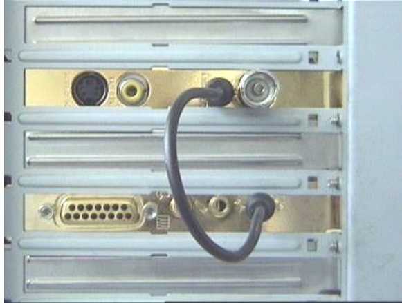
fig. 2: Connect the TV and sound card as illustrated here.
